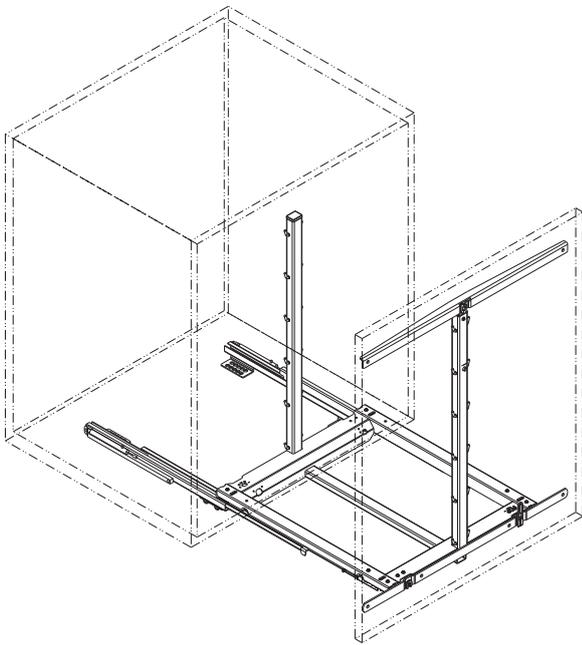
**LB** = Clear inside carcase width:  $\geq$  carcase width **B**-40 mm
