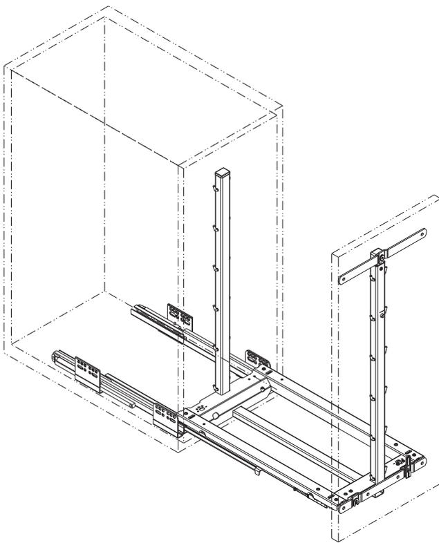
**LB** = Clear inside carcass width:  $\geq$  carcass width **B-32/38** mm
