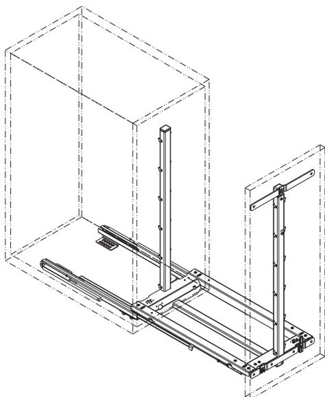
**LB** = Clear inside carcase width:  $\geq$  carcase width **B**-40 mm
